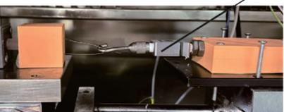
(a) Vertical adhesion test fixture
