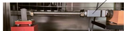
(b) Shear adhesion test fixture
