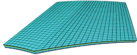
Fig.2 Mesh model of electro-thermal windshield
