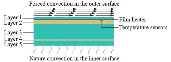
Fig.1 Typical configuration of electro-thermal windshield
