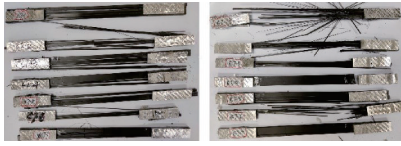
Fig.5 Damage morphology of specimens under high and low temperature cycle-humidity load coupling effect
