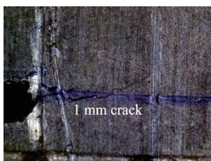
Fig.11 1 mm crack real magnification
