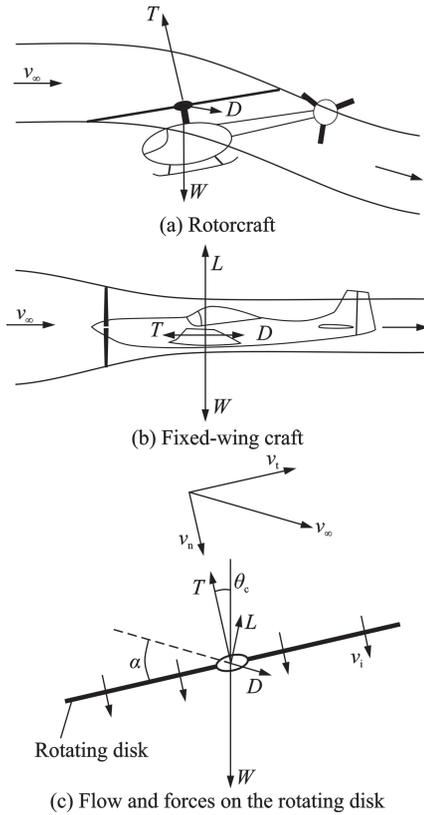
Fig.5 Aerodynamic models of aircraft
