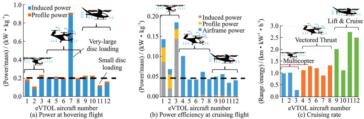
Fig.7 Flight performance of 12 eVTOL aircraft
