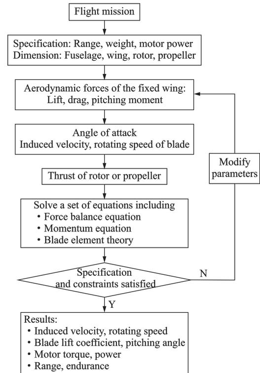
Fig.4 Synthesis process of performance estimation
