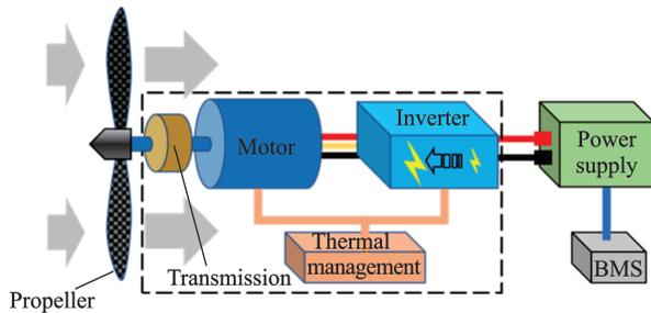
Fig.3 Rotor system of electric propulsion
