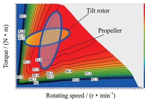
Fig.9 Representative efficiency map of motor
