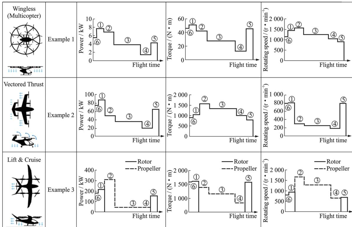
Fig.8 Examples of flight profile of motor output
