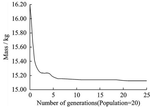
Fig.10 Convergence process for the size optimization of the bevel gear spoke plate
