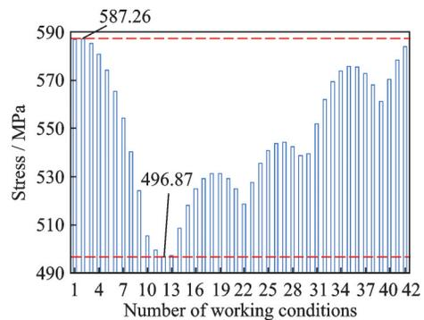
Fig.8 Maximum von Mises stress of the bevel gear spoke plate under 42 loading conditions after topology reconstruction
