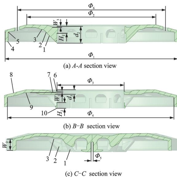
Fig.7 Section view of the parametric reconstruction model of the tilting prop bevel gear spoke plate
