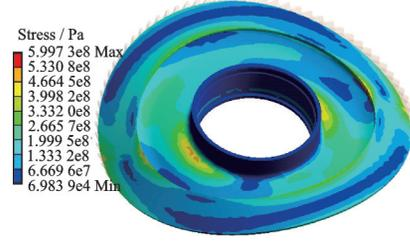
Fig.2 Stress contour plot of the initial gear spoke plate
