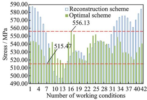
Fig.12 Comparison of the maximum stress of the spoke plate under 42 conditions before and after size optimization
