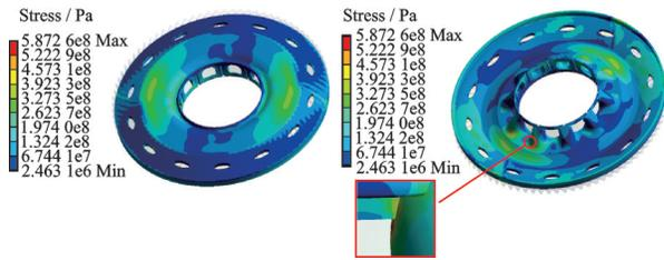
Fig.9 Stress contour plot of the bevel gear spoke plate under condition 2 after topology reconstruction
