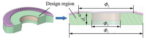
Fig.3 Half cycle symmetric model of the bevel gear with expanded design domain
