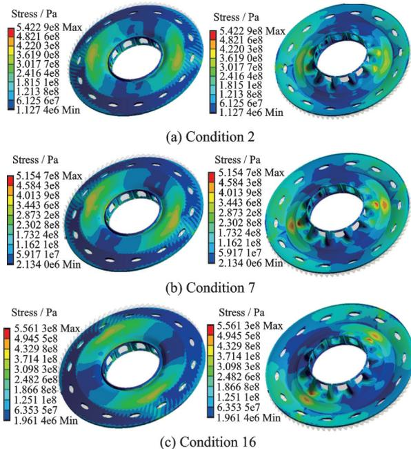
Fig.13 Stress contour plot of the bevel gear spoke plate under typical conditions after size optimization
