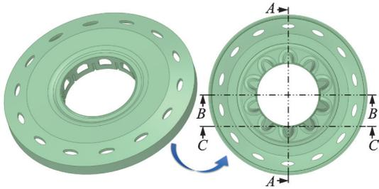
Fig.6 Parametric reconstruction model of the spoke plate of the tilting prop bevel gear
