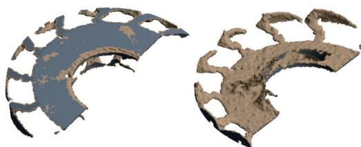
Fig.5 Bevel gear spoke plate after topology optimization
