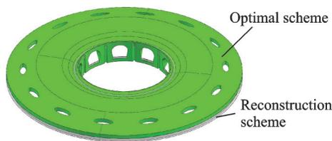
Fig.11 Comparison of bevel gear spoke plate structure schemes before and after size optimization
