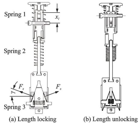
**Fig.6** Analysis of operating force of length adjusting component
