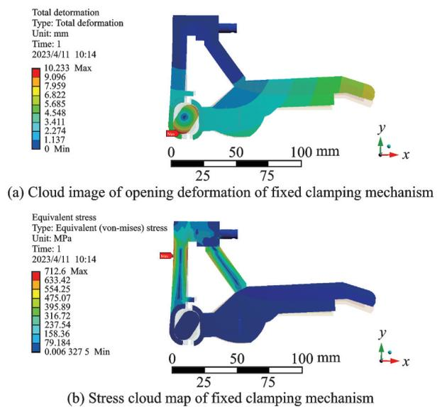
Fig.10 Deformation and stress cloud diagram of fixed clamping mechanism
