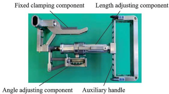
Fig.11 Engineering prototype of the extravehicular movable handrail
