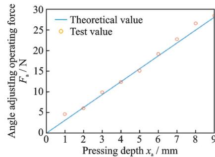
(b) Theoretical and measured values of angle adjusting operating force  $F_a$
