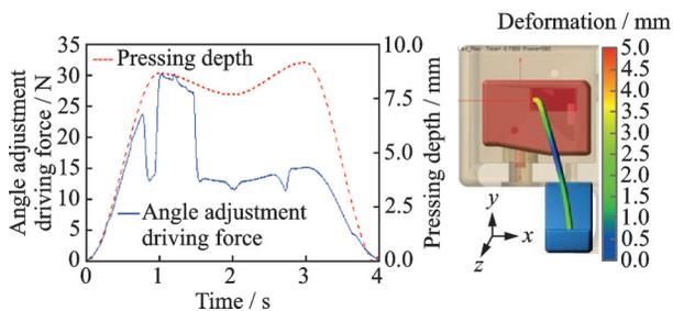
Fig.9 Analysis of angle adjustment driving force and rigid-flexible coupling dynamic model
