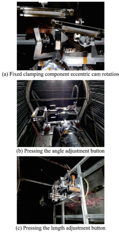
Fig.14 Thermal vacuum environment test
