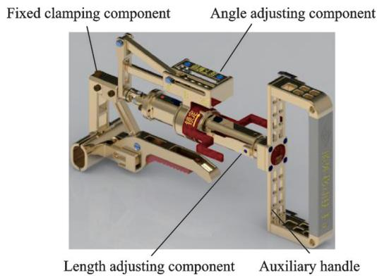
Fig.1 Structure diagram of the extravehicular movable handrail
