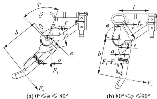
Fig.4 Operating force analysis of fixed clamping component
