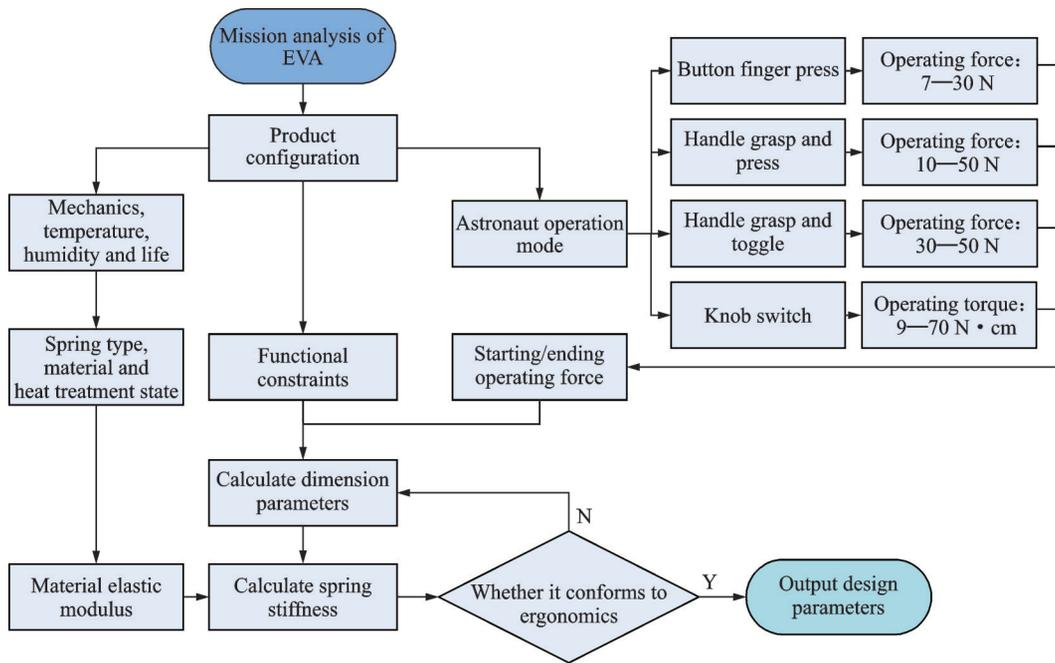
Fig.3 Operating force/moment design flow
