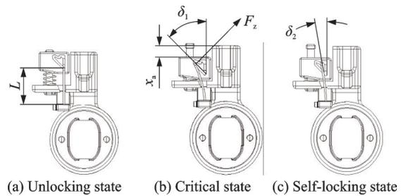
Fig.5 Analysis of operating force of angle adjusting component
