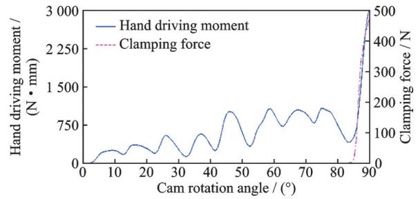
Fig.7 Analysis of hand driving moment and clamping force of fixed clamping component
