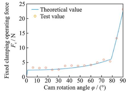
(a) Theoretical and measured values of fixed clamping operating force  $F_c$
