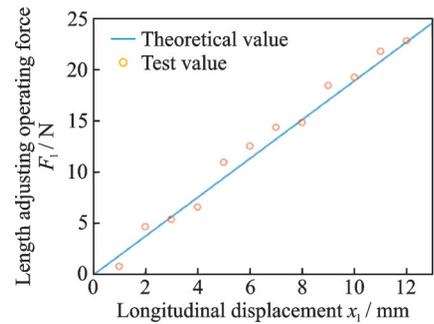
(c) Theoretical and measured values of length adjusting operating force  $F_l$
