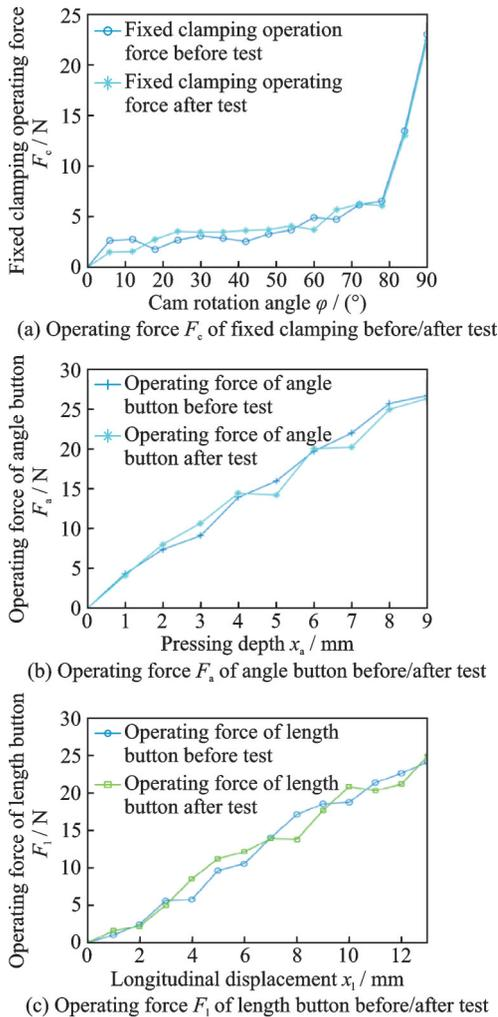
Fig.13 Operating forces before/after test
