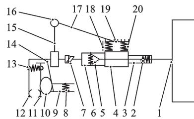
1—Auxiliary handle; 2—Bevel pin self-locking mechanism; 3—Inner rod; 4—Rack base; 5—Bevel pin mechanism; 6—Outer rod; 7—Cardan; 8—Pawl compression spring; 9—Pawl; 10—Eccentric cam; 11—Movable clamp; 12—Fix clamp; 13—Drag spring; 14—Ratchet wheel; 15—Strut; 16—Pin shaft; 17—Connecting rod; 18—Wire spring self-locking mechanism; 19—Rack; 20—Rack compression spring
