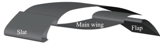
Fig.7 Geometry model of multi-element airfoil
