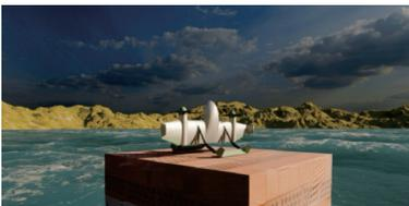
Fig.2 Conceptual diagram of the tail-sitter VTOL UAV incorporating free-tail in takeoff / landing state
