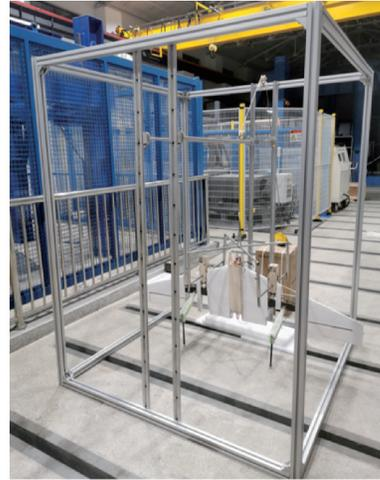
(b) Prototype of tail-sitter VTOL UAV drop test bench
