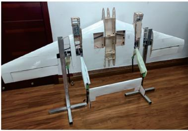
Fig.13 Tail-sitter VTOL UAV incorporating free-tail bionic technology
