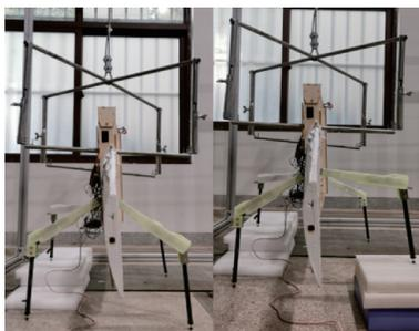
Fig.15 Landing test of tail-sitter VTOL UAV landing gear
