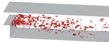
Fig.7  $Q=1.7e-6$  iso-surface calculated by SATES when the number of cells is 3 million
