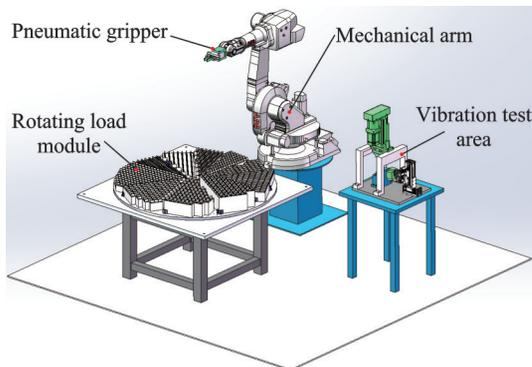
Fig.2 3D design of hardware platform for blade natural frequency test
