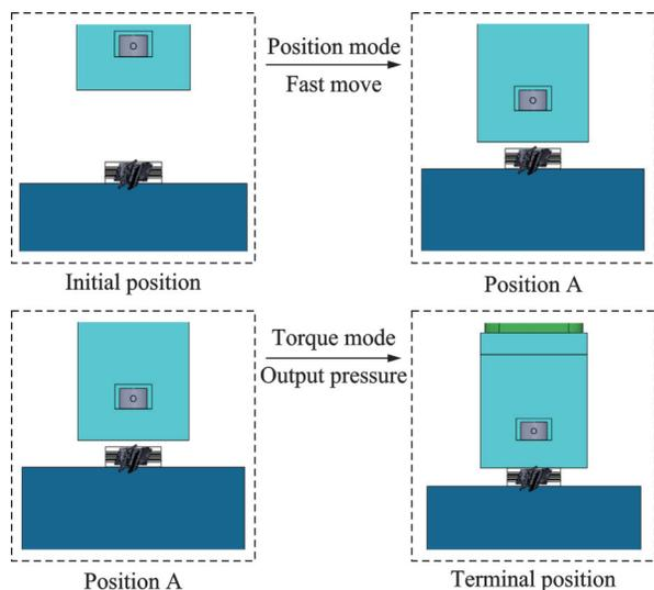
Fig.5 Motion diagram of servo electric cylinder
