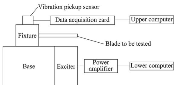
Fig.1 Principle diagram of blade natural frequency testing
