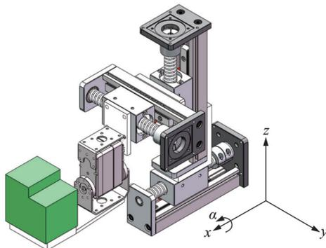
Fig.10 Four-dimensional motion platform equipped with exciter
