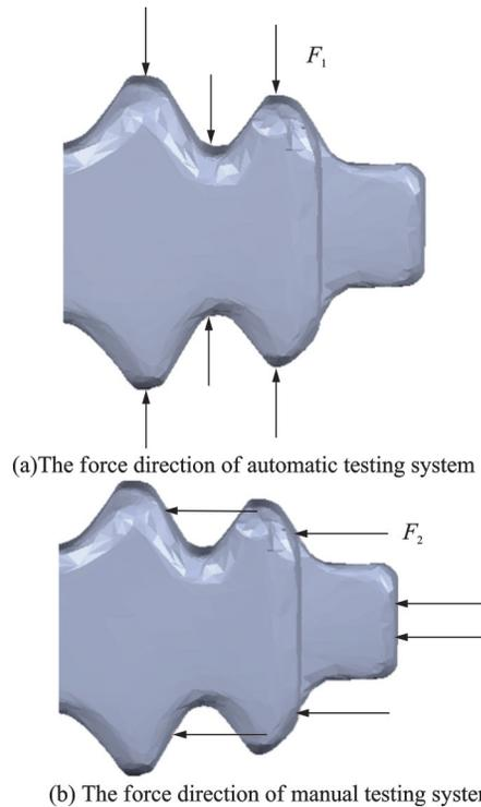
Fig.16 Difference of clamping force application modes between two test systems
