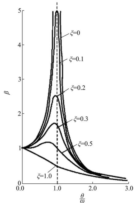
Fig.12 System frequency response curves
