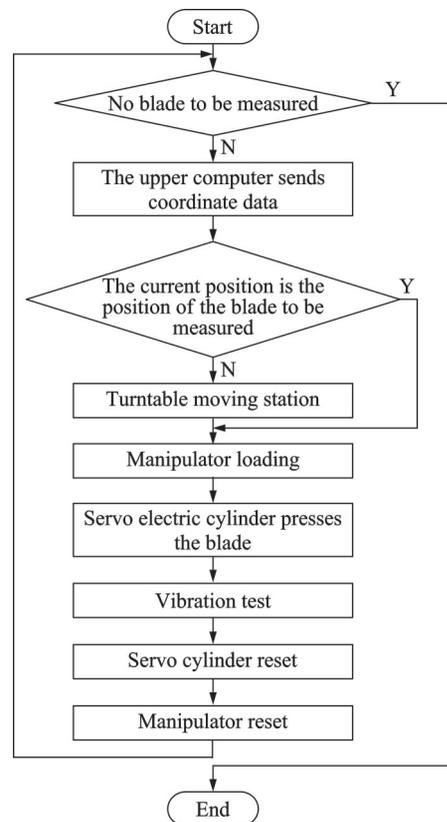
Fig.4 Motion control flow of blade natural frequency test
