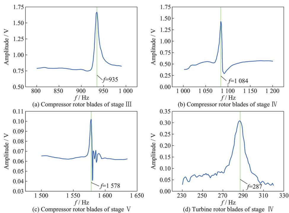
Fig.14 Partial amplitude-frequency response curves of accuracy experiment
