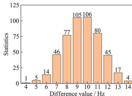
Fig.17 Statistics of natural frequency difference of two test systems
