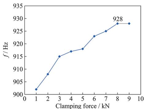
Fig.8 Relation between the clamping force and natural frequency of the compressor rotor blades of stage II
