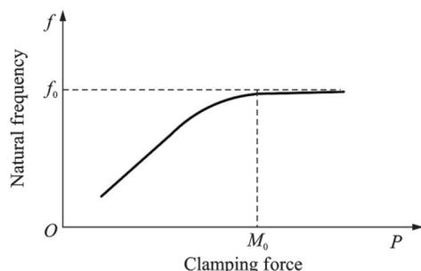
Fig.6 Relation between clamping force and frequency
