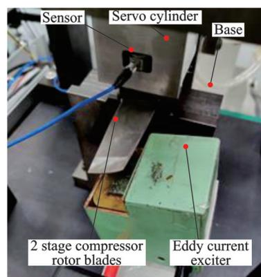
Fig.7 Test of compressor rotor blades of stage II
