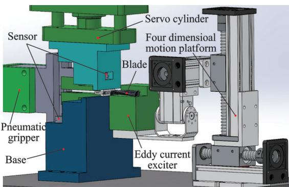
Fig.3 3D design of the test area
