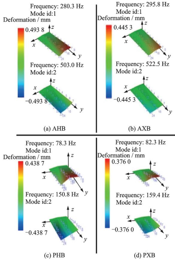
Fig.16 EMA mode shapes of aluminum , PLA material hollow and BCC blades
