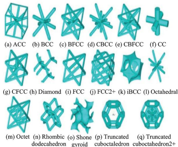
Fig.1 Examples of lattice structure unit cells<sup>[2]</sup>
