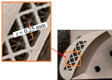
Fig.3 Metallic turbine blade with octet truss lattice of 0.25 mm strut thickness
