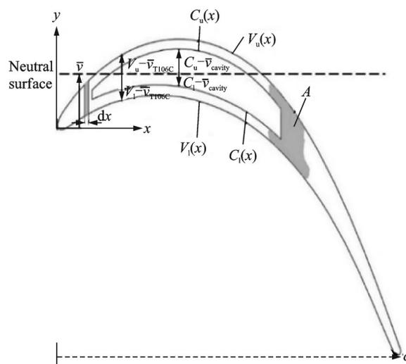
Fig.4 Quantities for determining and estimating the bending inertia of a hollow airfoil section
