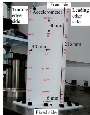
Fig.11 Measurement points of the blade
