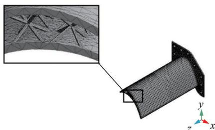
Fig.13 BCC blade meshed model
