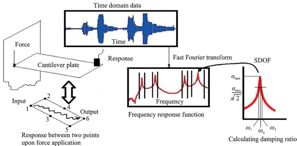
Fig.10 Experimental modal testing and analysis
