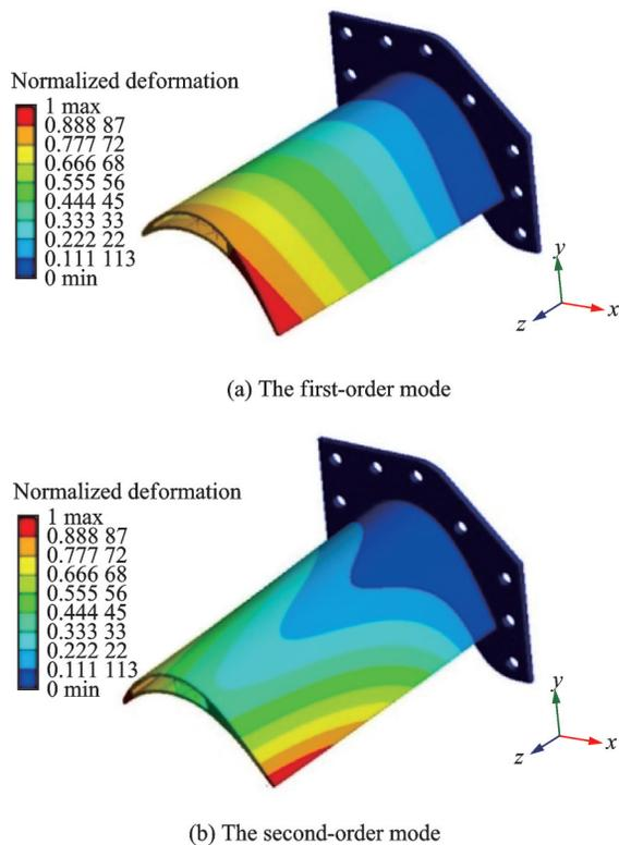
Fig.18 Mode shapes for the BCC blade
