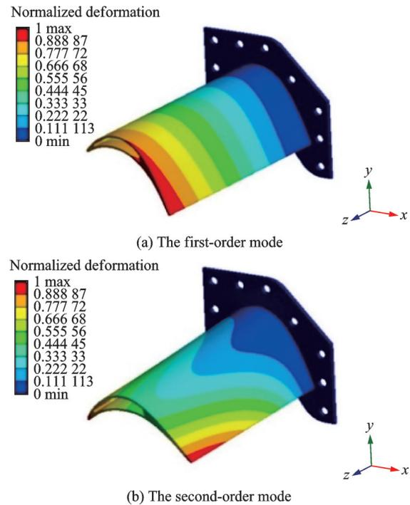
Fig.17 Mode shapes for the hollow blade
