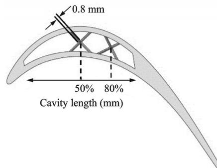
Fig.7 Hexagonal strut BCC lattice structure at 50% and 80% of the cavity length
