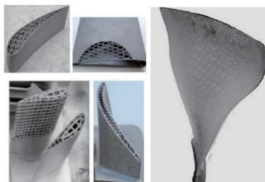
(b) Portions of printed lattice structures in blades
