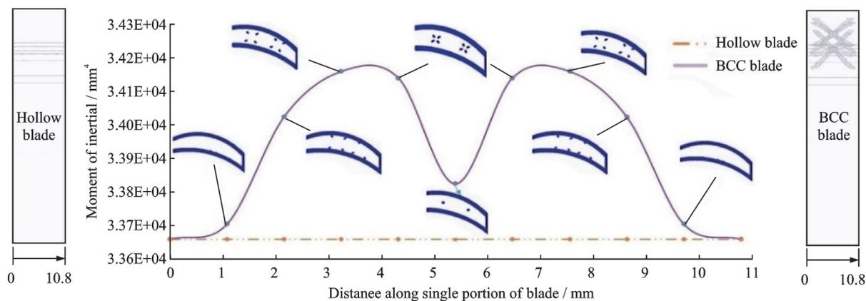
Fig.8 Moment of inertia of hollow and BCC blade of a 10.8 mm portion
