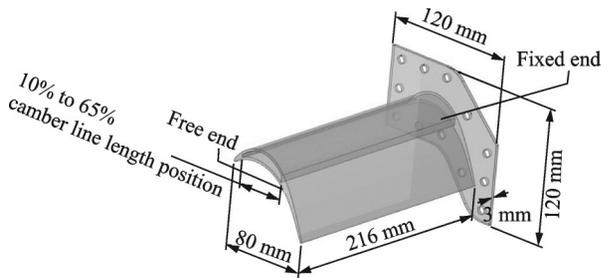
Fig.5 Dimensions of hollow blade geometry with base plate
