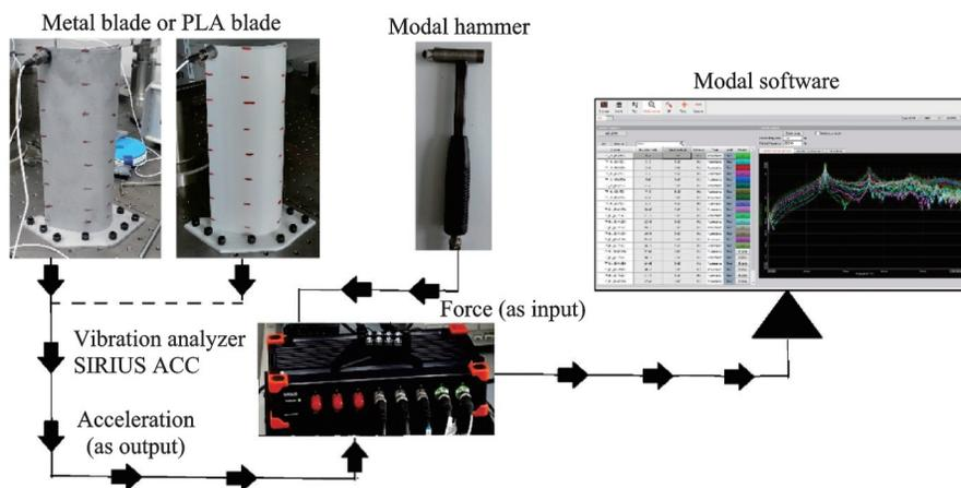
Fig.12 Experimental modal testing flow chart
