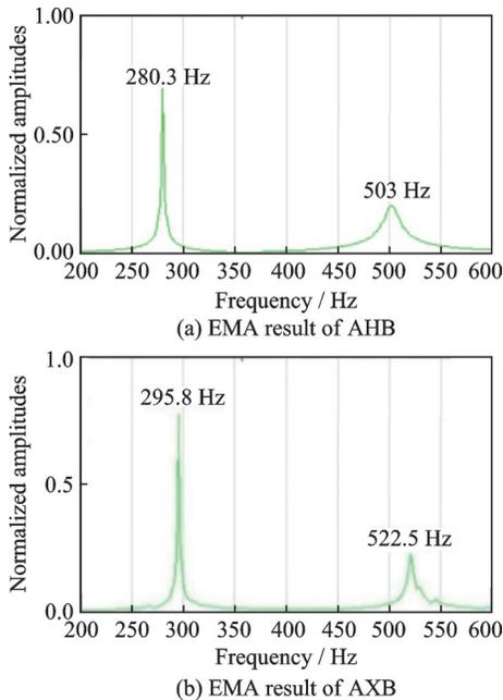
Fig.14 Natural frequencies of aluminum alloy blade
