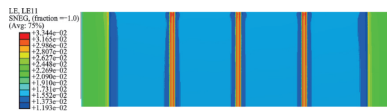
Fig.8 Simulation results of thin film arrays in the X direction
