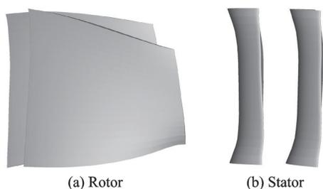
Fig.12 Forward-swept rotor and curved stator
