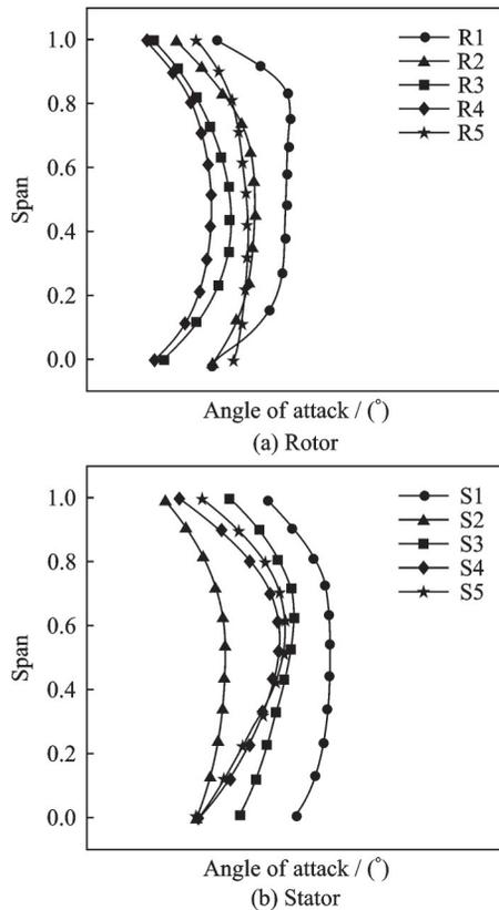
Fig.3 Angle of attack distribution
