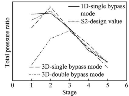
Fig.4 Stage pressure ratio distribution of different working modes
