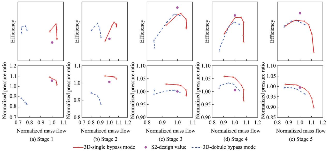
Fig.5 Predicted stage matching characteristics for two working modes
