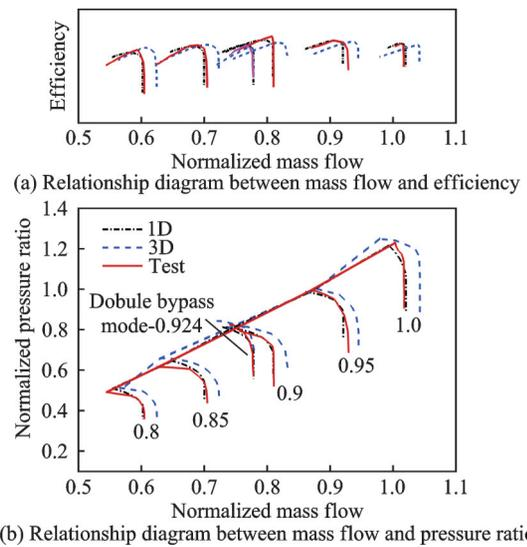
Fig.15 Comparison of total performance test characteristics and design characteristics
