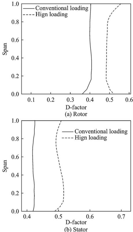
Fig.10 Diffusion factor distribution of high-load and conventional load compressors
