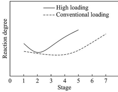
Fig.9 Stage reaction degree distribution of high-load and conventional load compressors
