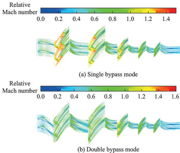
Fig.13 Relative Mach number distribution at 90% blade height section for different working modes
