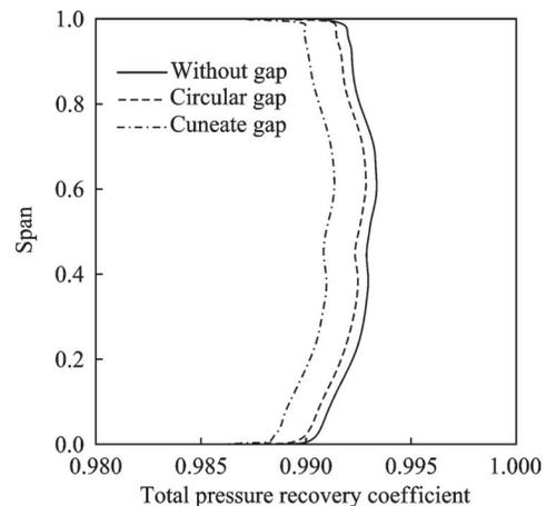
Fig.7 Total pressure recovery coefficient comparison between three gap structures
