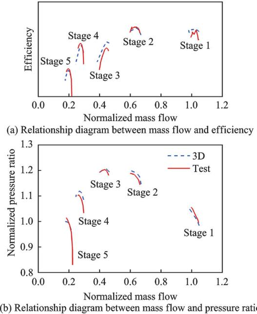
Fig.17 Stage characteristics and simulation results for double bypass mode
