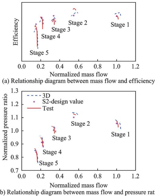
Fig.16 Stage characteristics and simulation results for single bypass mode
