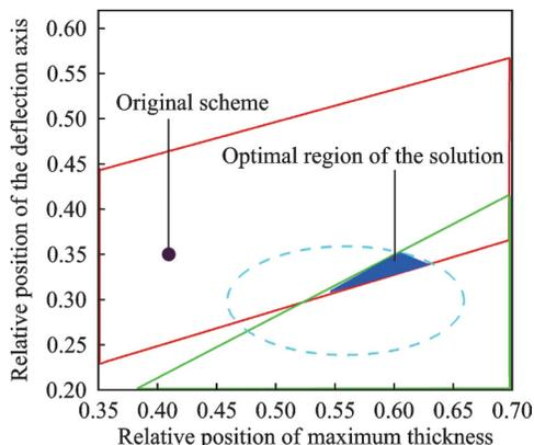
Fig.8 Optimization of design parameters
