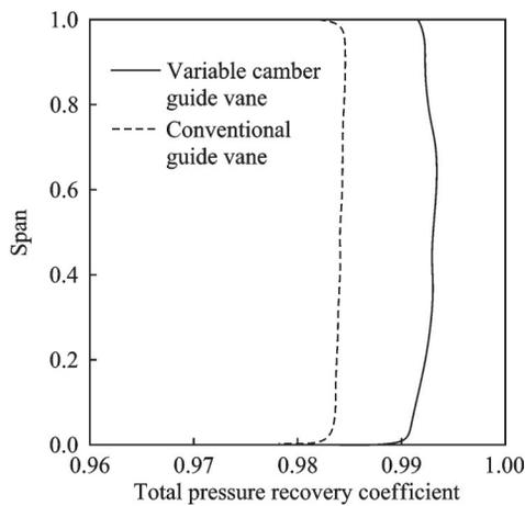
Fig.6 Comparison of total pressure recovery coefficient between variable camber guide vane and conventional guide vane
