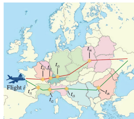
Fig.3 Schematic diagram of assigning delay and alternative trajectory option
