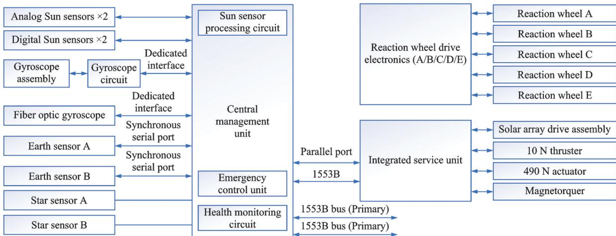
Fig.5 Composition of the Beidou-3 IGSO Satellite ADCS
