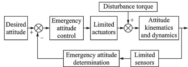
Fig.1 Structural of the satellite ADCS system in emergency mode
