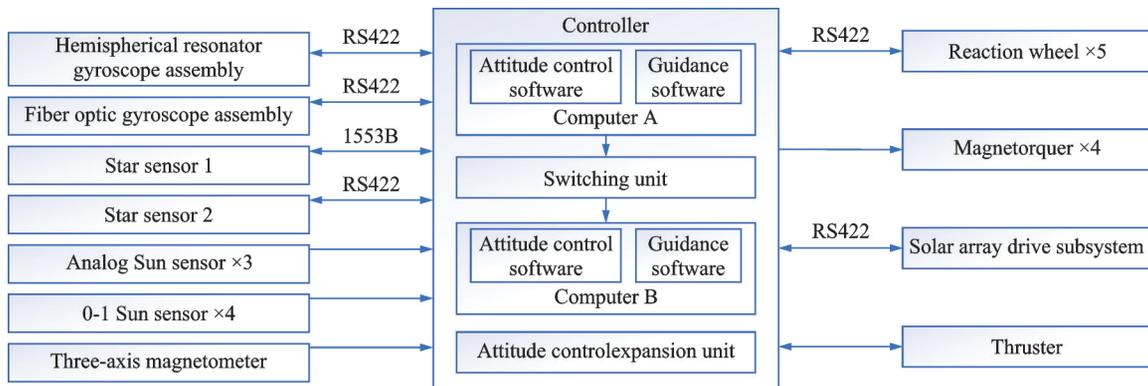
Fig.4 Composition of the Atmospheric Environment Monitoring Satellite ADCS
