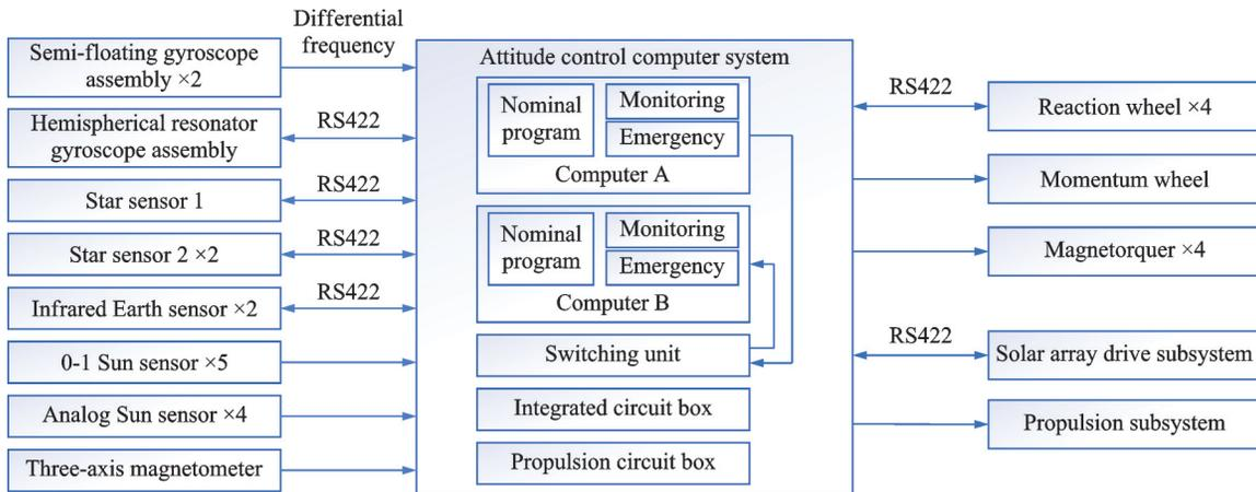
Fig.3 Composition of the Gaofen-5 Satellite ADCS
