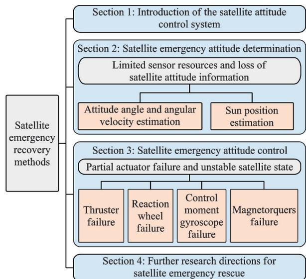
Fig.2 Structure of satellite emergency recovery methods
