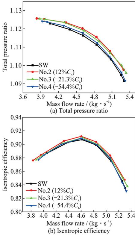
Fig.7 Experimental compressor performance curves for different injection axial positions
