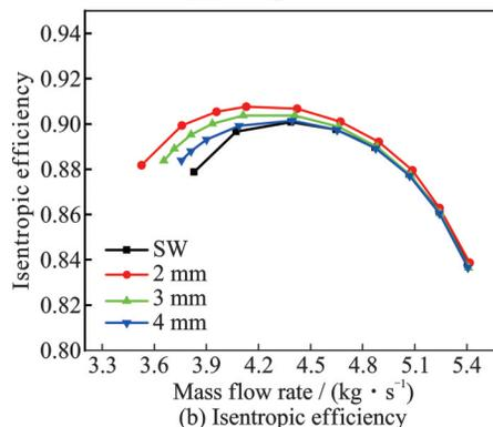
Fig.18 Numerical compressor performance curves for different injector diameters
