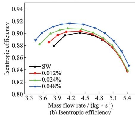
Fig.14 Numerical compressor performance curves for different injected mass flow rates
