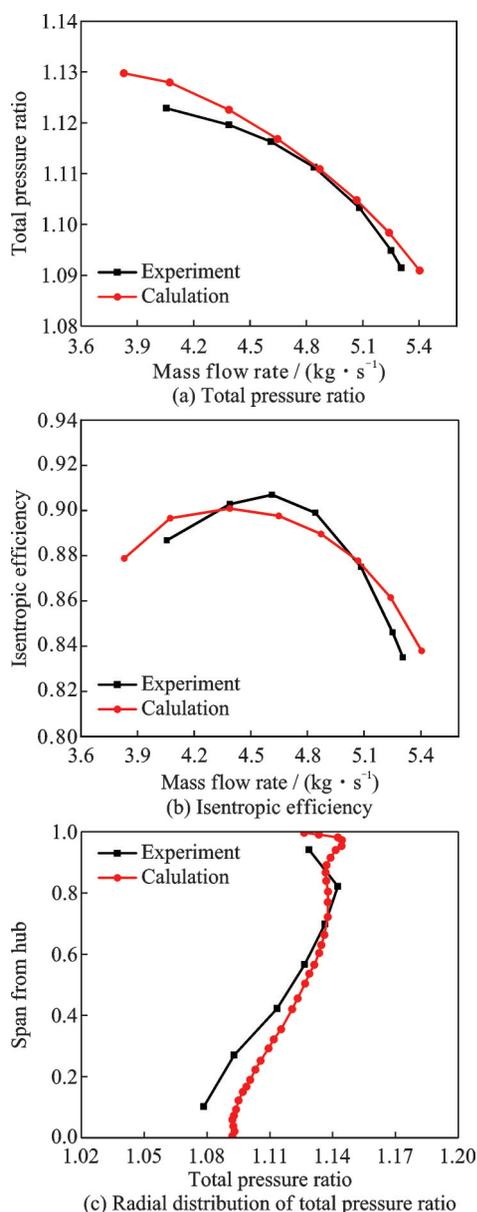
Fig.4 Comparison between numerical and experimental results
