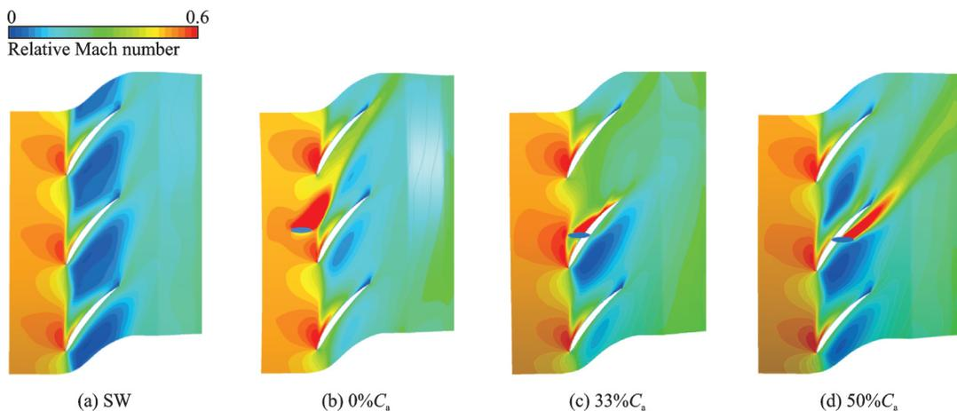
Fig.11 Distribution of the relative Mach number at 99% blade span for different injection axial positions under near-stall condition
