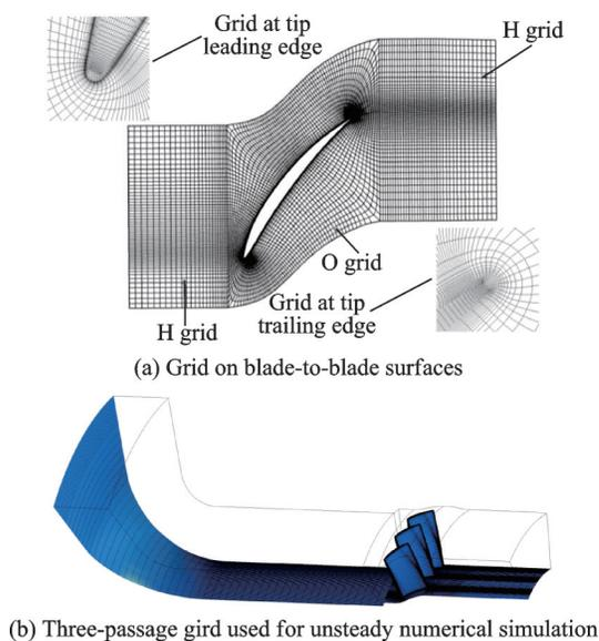
Fig.3 Grid diagram of calculation domain
