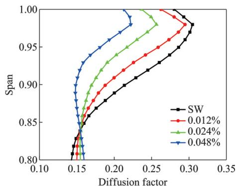
Fig.17 Radial distribution of the diffusion factor for different injected mass flow rates under near-stall condition
