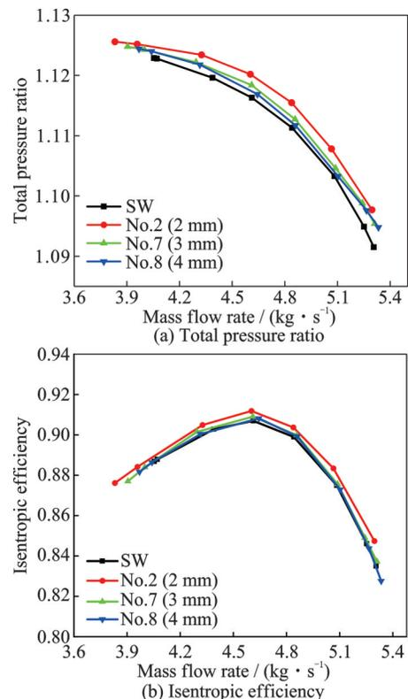
Fig.9 Experimental compressor performance curves for different injector diameters
