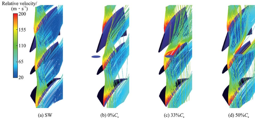
Fig.12 Distribution of tip leakage flow streamline for different injection axial positions under near-stall condition
