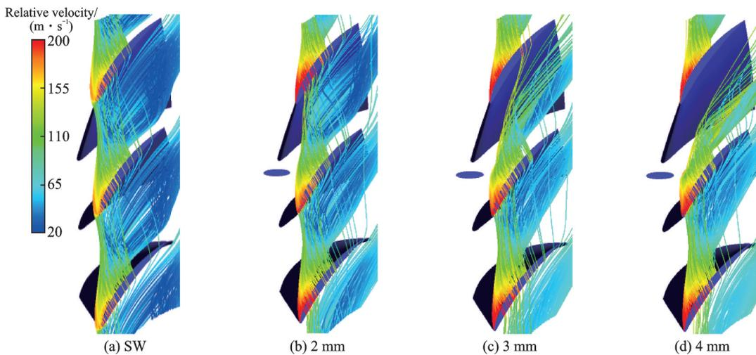
Fig.20 Distribution of tip leakage flow streamline for different injector diameters under near-stall condition
