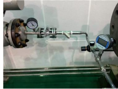
(b) Pressure reducing valve and pressure gauge
