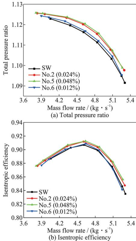
Fig.8 Experimental compressor performance curves for different injected mass flow rates
