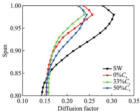
Fig.13 Radial distribution of the diffusion factor for different injection axial positions under near-stall condition
