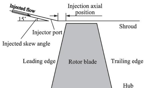
Fig.5 Diagram of the micro tip injection structure
