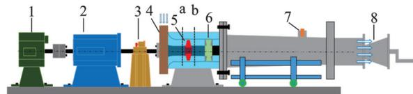
1—DC motor; 2—Accelerator; 3—Torque meter; 4—Intake steel cover; 5—Rotor disk; 6—Stator disk; 7—Orifice flowmeter; 8—Throttle valve; a—Rotor inlet probe location; b—Rotor outlet probe location
