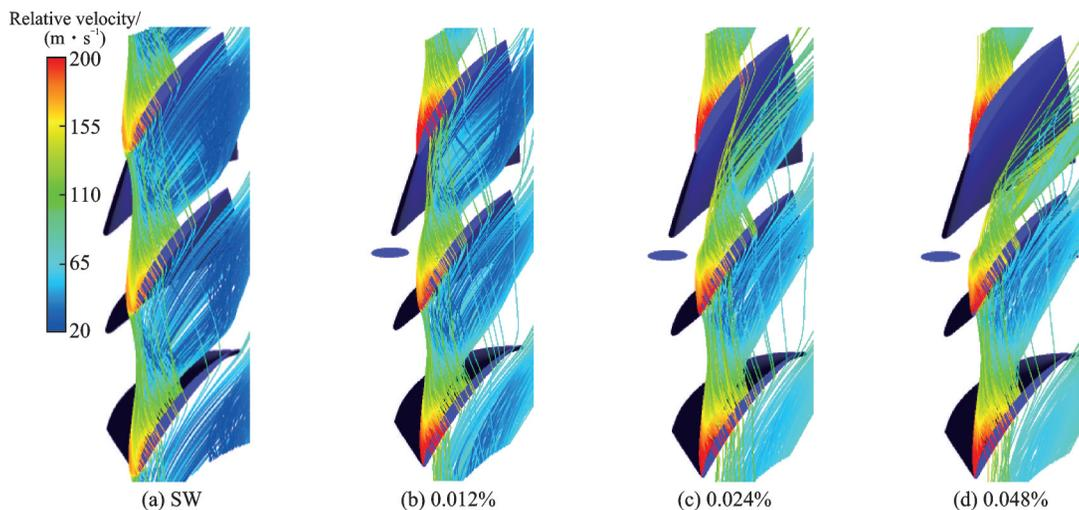
Fig.16 Distribution of tip leakage flow streamline for different injected mass flow rates under near-stall condition
