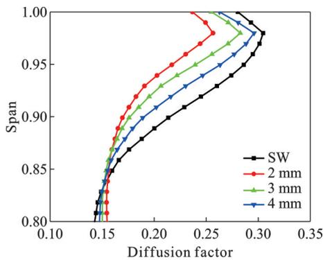
Fig.21 Radial distribution of the diffusion factor for different injector diameters under near-stall condition
