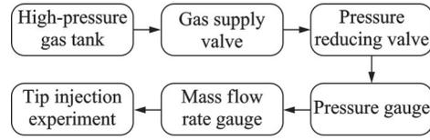
(a) Schematic diagram of gas transmission
