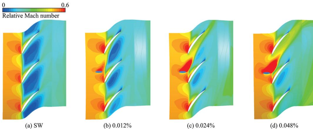
Fig.15 Distribution of the relative Mach number at 99% blade span for different injected mass flow rates under near-stall condition
