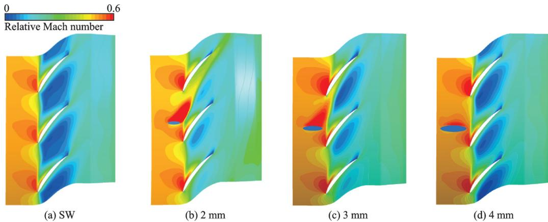
Fig.19 Distribution of the relative Mach number at 99% blade span for different injector diameters under near-stall condition
