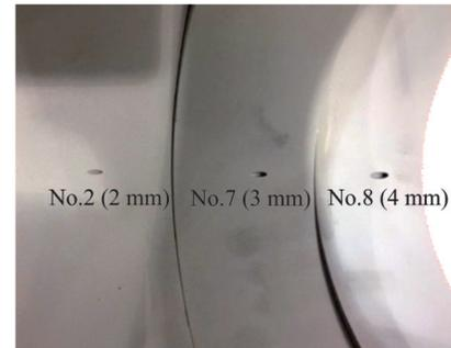
(d) Comparison of micro tip injection test pieces for different injector diameters
