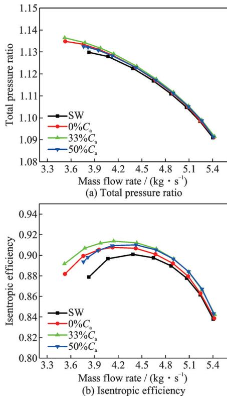
Fig.10 Numerical compressor performance curves for different injection axial positions
