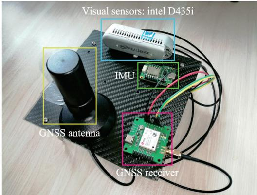
Fig.1 Tightly coupled multi-sensor state estimation platform
