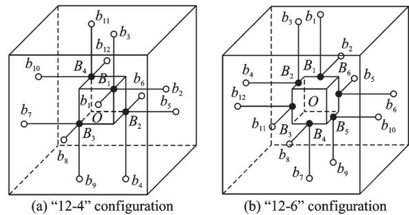
Fig.1 Principle prototype of parallel six-dimensional acceleration sensing mechanism
