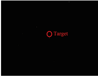
Fig.19 Simulated image with adding device noise
