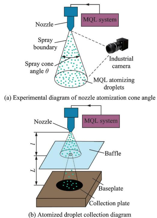
Fig.4 Experimental schematic diagram
