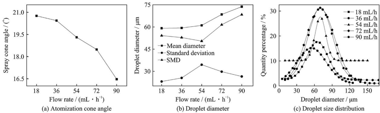
Fig.13 Influence of lubricating oil flow rate on atomization effect of nozzle
