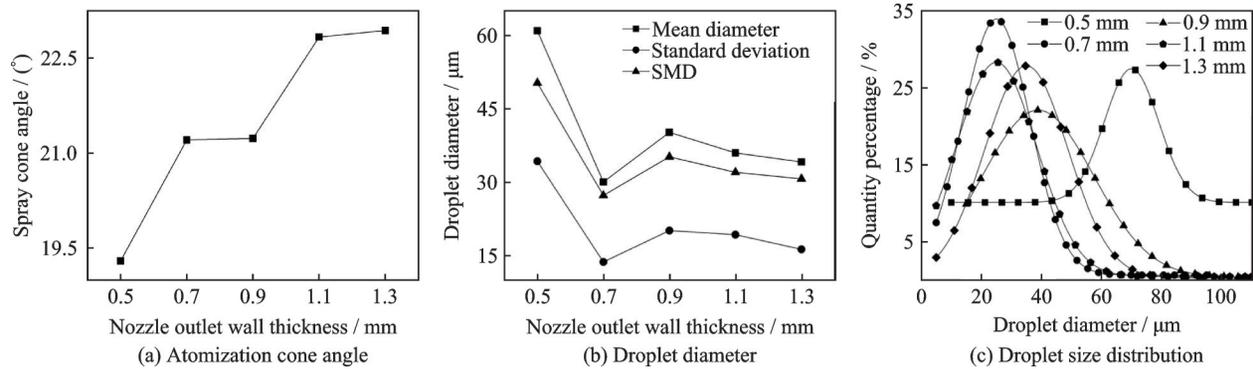
Fig.9 Influence of nozzle outlet wall thickness on atomization effect
