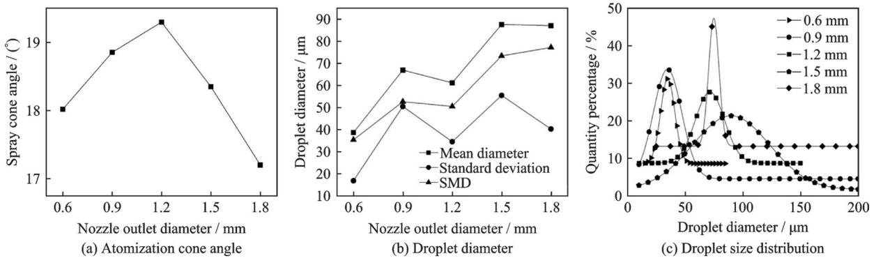
Fig.8 Influence of nozzle outlet diameter on atomization effect
