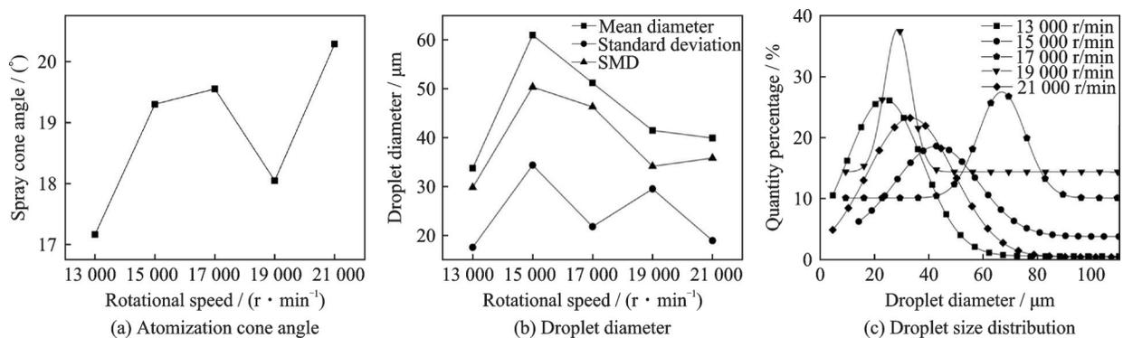
Fig.10 Influence of nozzle machining spindle speed on atomization effect
