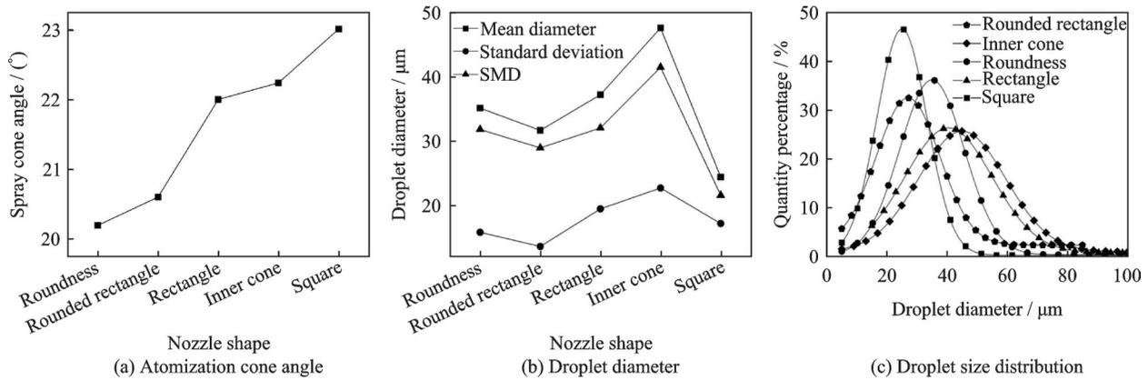
Fig.7 Influence of nozzle outlet shape on atomization effect
