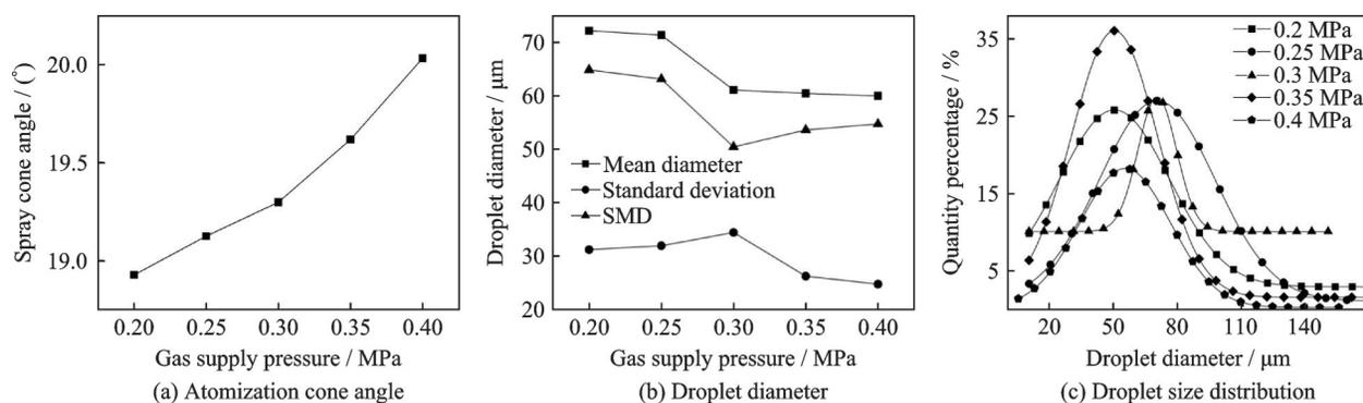
Fig.12 Influence of MQL gas supply pressure on atomization effect
