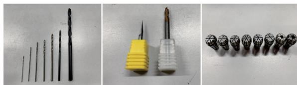
(a) HSS twist drill (b) Milling cutter (c) Elastic fixture
