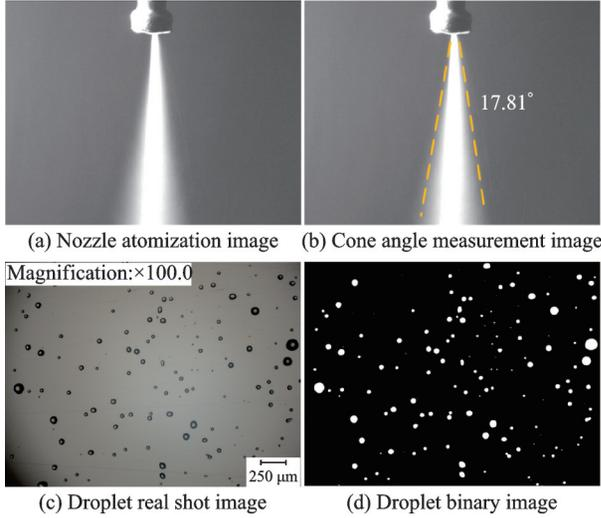
Fig.5 Atomization and droplet images
