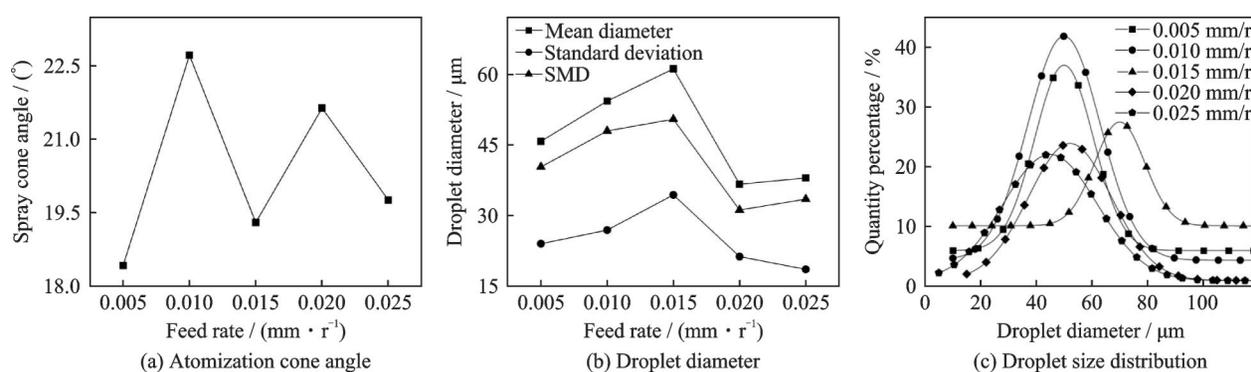
Fig.11 Influence of nozzle machining cutting tool feed rate on atomization effect
