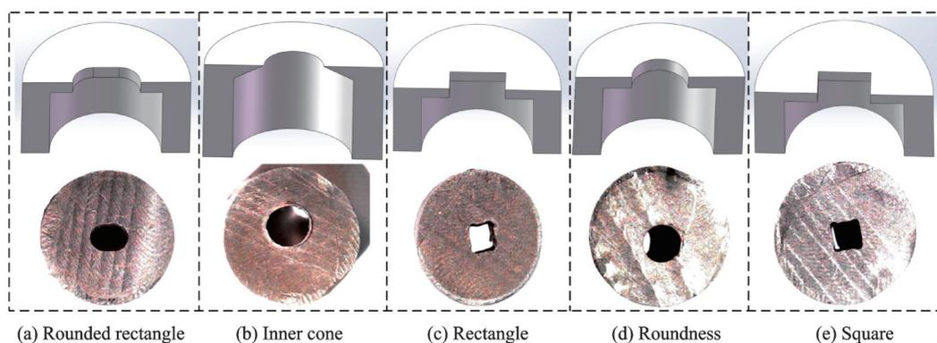
Fig.3 Three-dimensional and physical maps of MQL nozzle
