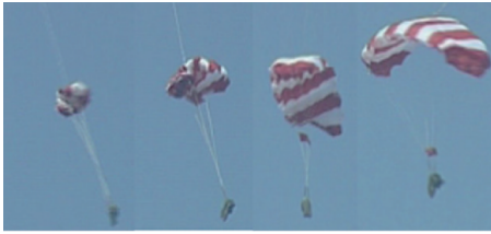
Fig.1 Opening process of parafoil system
