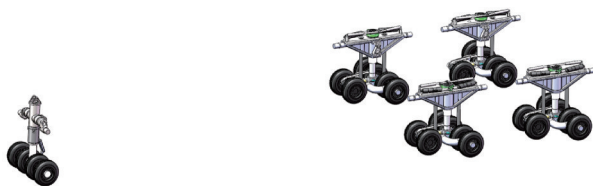
Fig.8 Schematic diagram of the C-5 steering kinematic model
