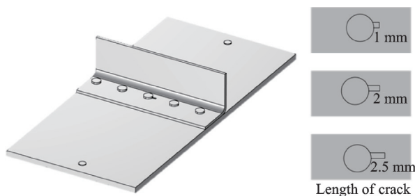
Fig.18 Conditions of crack application in multi-layer riveted structures
