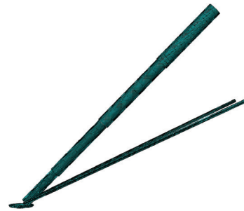
Fig.4 Finite element model of landing leg
