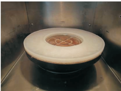
Fig. 2 Ice fixed abrasive pad with the original cast iron base
