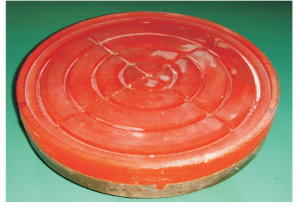
Fig. 3 Mold with Polyurethane heat-insulating layer
