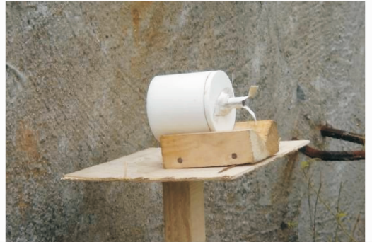
Fig. 9 Test site layout of \varnothing 60 mm shaped charge penetrating concrete
