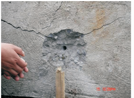
Fig. 12 In-crater of the third \varnothing 60 mm shaped charge
