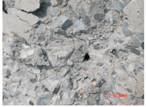
Fig. 10 In-crater of the first \varnothing 60 mm shaped charge
