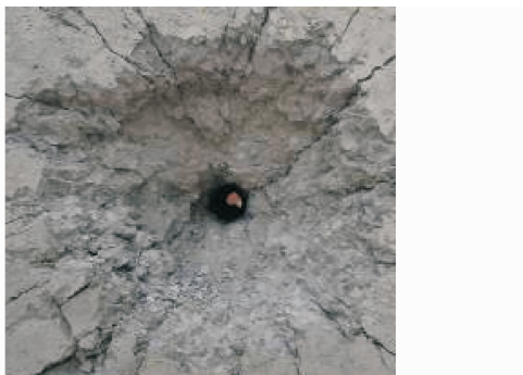
Fig. 13 In-crater of \varnothing 142 mm shaped charge
