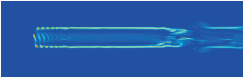
Fig. 14 Visualization of the vorticity contour in the Phase VI rotor wake
