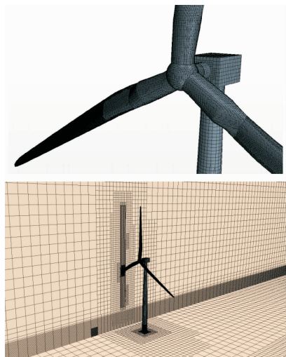
Fig. 3 Surface grid and mesh section
