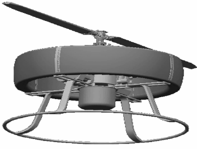
Fig. 1 Structure of coaxial rotor ducted fan helicopter
