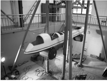
Fig. 4 Impact test for UAV airbag system
