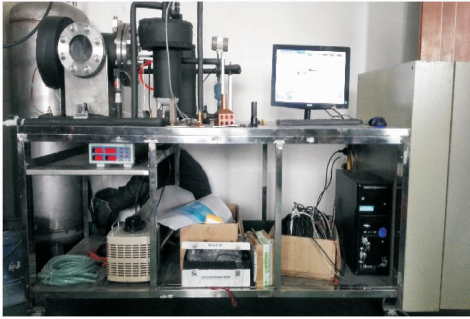
Fig. 4 Physical map of water spray cooling system
