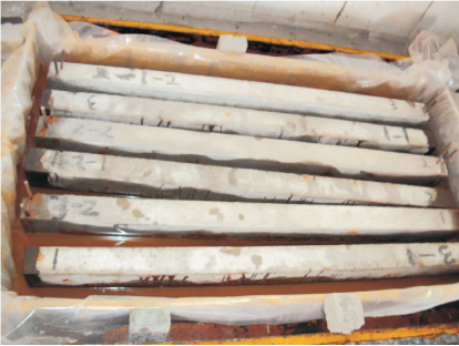
Fig. 2 Beam specimens being secondly-corroded
