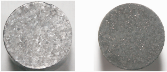
(a) Surface of Ti40 after ECM using sodium chloride (b) Surface of Ti40 after ECM using sodium nitrate electrolyte
