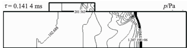
Fig. 4 Pressure contour in detonation chamber
