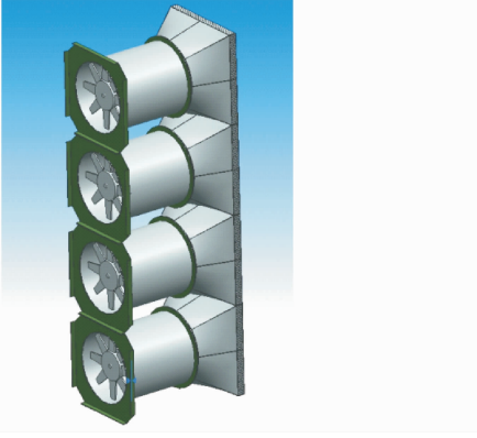
Fig. 2 Connections of the axial fans
