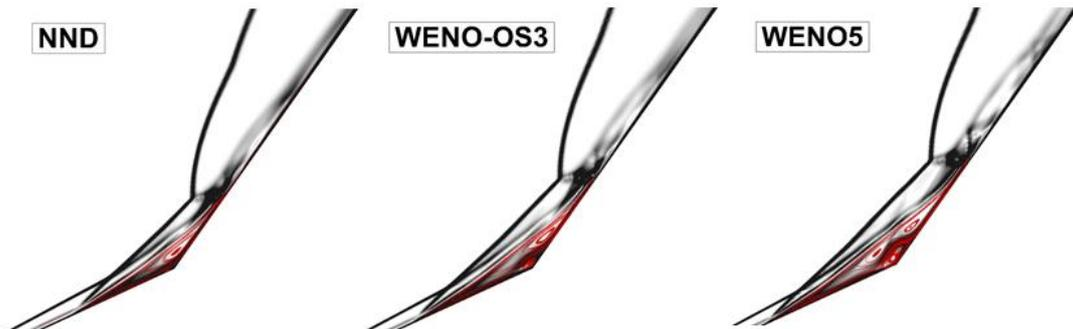
Fig. 3 Density gradient contours and separation region by different numerical schemes
