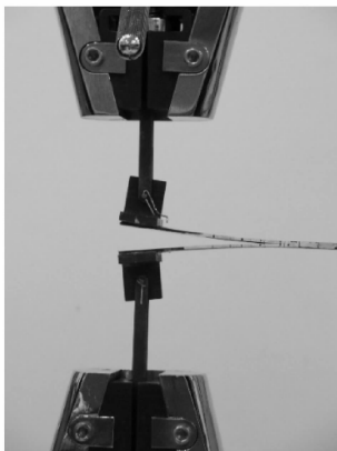
Fig. 6 Experiment fixture of DCB test
