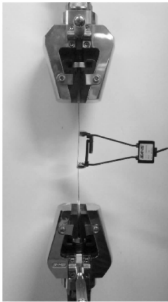
Fig. 5 Fixture of partly-cured Z-pin tensile test
