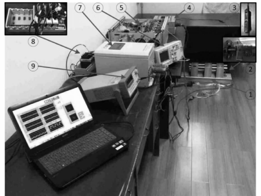
①—Test rig; ②—Fiber optic probe; ③—Fiber amplifier; ④—Current switch and control box; ⑤—PID control box; ⑥—Oscilloscope; ⑦—Drive; ⑧—Data acquisition; ⑨—Signal generator (a) Rotor-AMB system
