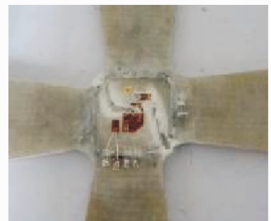
Fig. 2 Tensile failure form of cruciform specimen when biaxial loading ratio equals 1 [6]
