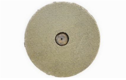
Fig. 4 Thermosetting fixed abrasive lapping pad
