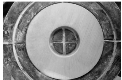
Fig. 3 Ice-fixed abrasive lapping pad
